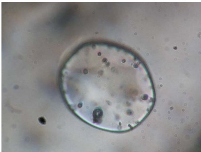
Fig 10. Sample R-82. Similar melt inclusion with gas bubbles in Quartz, rhyolite, East Bazman volcano, T = 630oC. After next T = 690oC gas bubbles will disappear. H 2 O content is up to 6 wt%.
