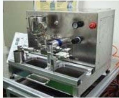
High Pressure Homogenizer (NANO- H5)
