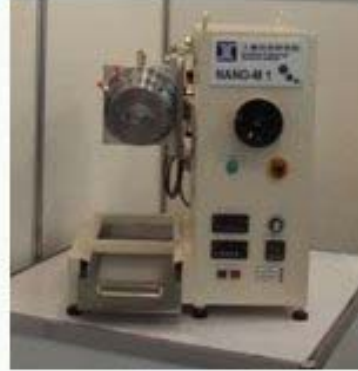
Grinding Dispersing Equipment (NANO-M1)
