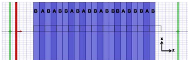
Figure 2 1-dimensional SbSI based Fibonacci photonic crystal structure (FPCs).
