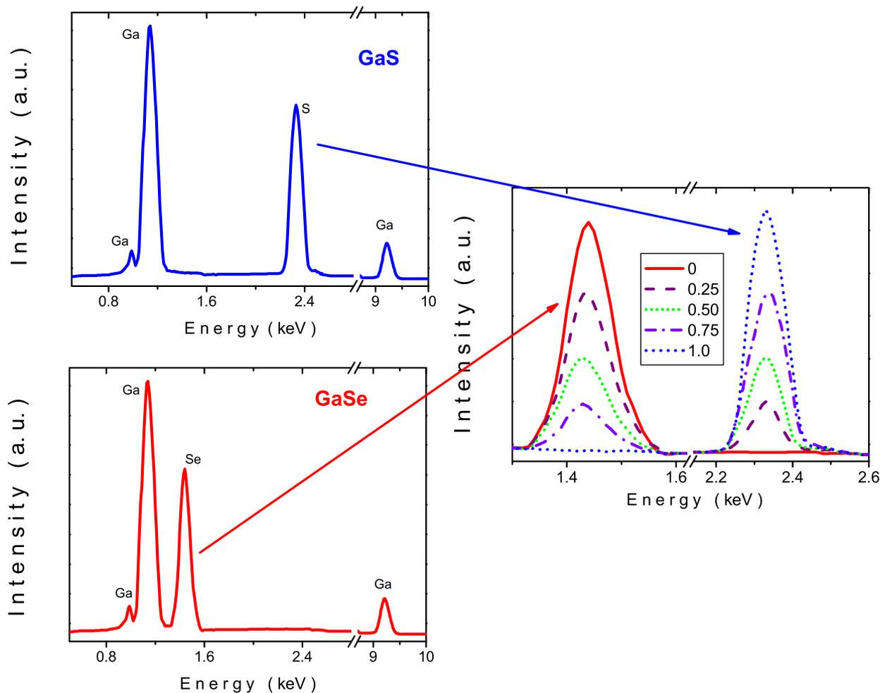
Fig. 1. Energy dispersive spectroscopic analysis of  $\text{GaS}_x\text{Se}_{1-x}$  mixed crystals.
