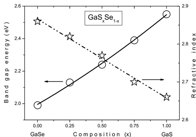
**Fig. 5.** Compositional dependences of the refractive index and the energy band gap in GaS<sub>x</sub>Se<sub>1-x</sub> mixed crystals. The solid and dashed-dotted lines show the fitted line according to Eq. (4) and linear fit, respectively.
