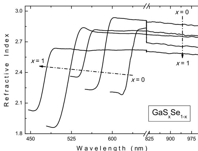
**Fig. 4.** The dependences of the refractive index on the wavelength for different compositions of GaS<sub>x</sub>Se<sub>1-x</sub> mixed crystals.
