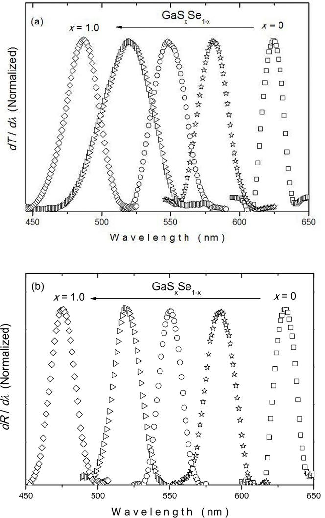
Fig. 3. The dependence of (a)  $dT/d\lambda$  and (b)  $dR/d\lambda$  on photon energy for  $\text{GaS}_x\text{Se}_{1-x}$  mixed crystals.
