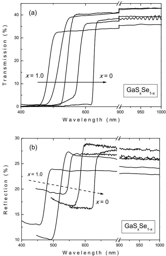
Fig. 2. The spectral dependence of (a) transmission and (b) reflection for  $\text{GaS}_x\text{Se}_{1-x}$  mixed crystals.
